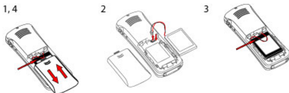
Figure 10: Battery replacement
